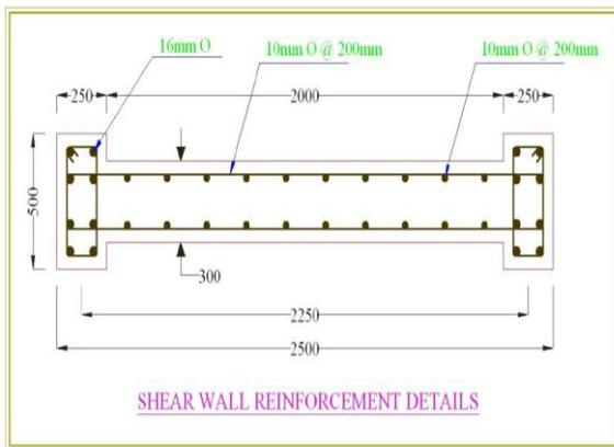
Figure 7.1 Reinforcement details of shear wall
