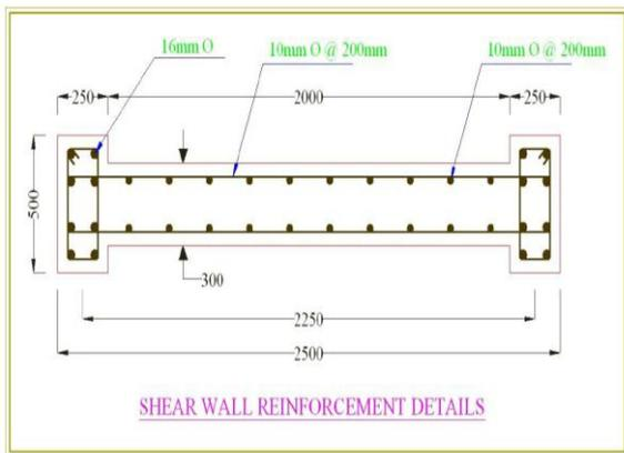
Figure 7.1 Reinforcement details of shear wall
