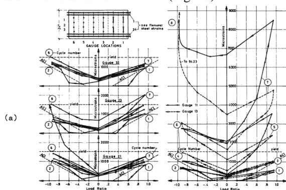
Fig. 4.1. The Load-Strain relationship for the (a) stirrups
