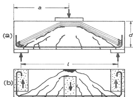
Fig 3.1 Arch Action as Affected by the Introduction of Load into a Beam.
