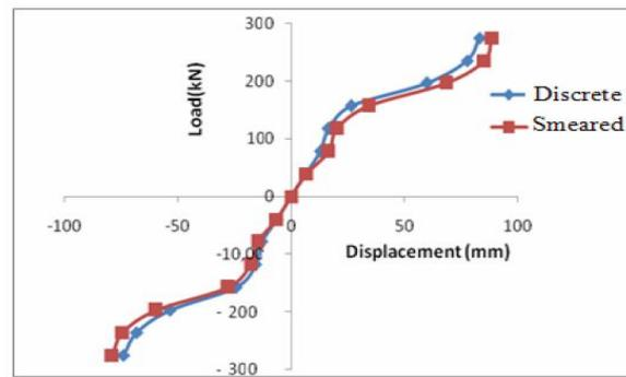
Figure 9.1 Load - displacement envelope curve for models
