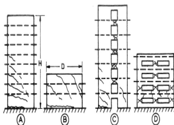
Fig.5.1 Vertical web reinforcement in shear walls
